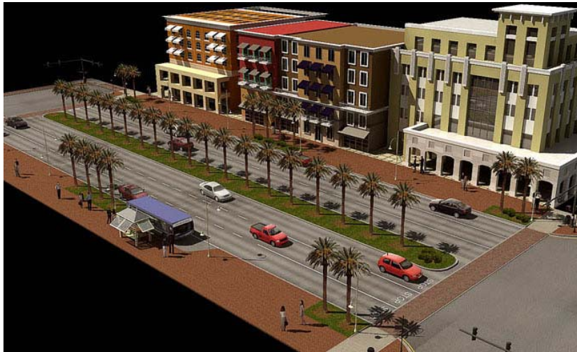
The proposed future condition of SR 7 showing buildings pulled up to the street, wide sidewalks, bricked crosswalks, pedestrian scale lighting, landscaping, pull-outs for bus rapid transit, and maintenance of the existing six-lane street section
